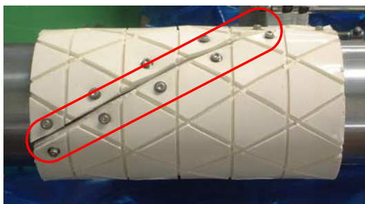
Figure 9. Parallelogram-shaped silicone rubber female mold.
